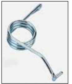
Above: The tiny brake spring that failed and needed to be replaced.
