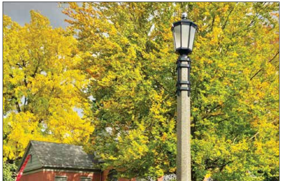
Light poles have been replaced at many Portland parks, including 65 at Irving Park and 10 at Montavilla Park. Work began in May to replace 88 poles at Mount Tabor Park, above. The project improved faulty anchoring and the installation of environmentally friendly LED lights.
