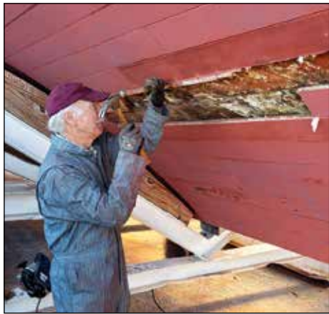
Steve Stange repairs damaged mahogany planks as he helps restore a U.S. Navy PT boat on Swan Island. (Michael Wright)
